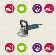
Handheld Grinders for Mortar Removal 25 CFM / INCH OF WHEEL DIAMETER
